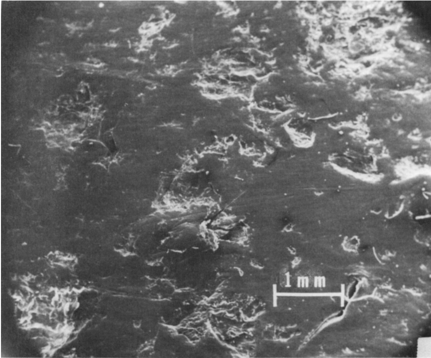
Fig. 2. Another typical clinical wear surface, also after eight months of service.
