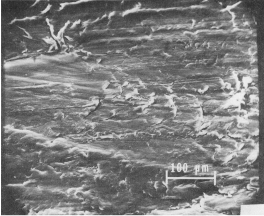
Fig. 1. Typical UHMWPE articular surface as seen in the scanning electron microscope. This prosthesis has been implanted and used ca. eight months.
